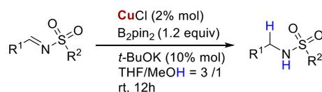
Scheme 2. Transfer hydrogenation of sulfonyl imines catalyzed by first-row transition metals.
